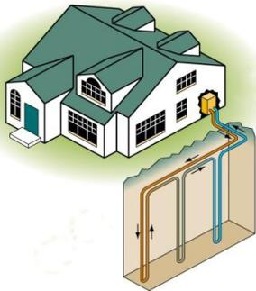
ground-source—heat pumps (GHPs) circulate water through a closed loop of plastic pipe that is inserted into vertical boreholes or laid out horizontally in relatively shallow trenches. The fluid discharges heat from a building into the ground during summer, and taps
